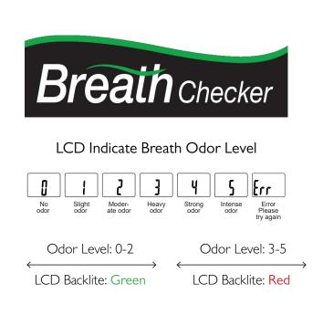
The HC-312F Breath Checker is an innovative palm-size monitor that detects and measures the presence of annoying or embarrassing breath odors. Simply turn it on, breathe into the sensor, and a reading appears on the digital display. Measures odor in seconds, with results displayed in six color coded levels.
