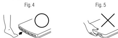
To recalibrate the scale, gently tap the Personal Key with your toe (see Fig.4). Do not place your hand on the scale while recalibrating (see Fig.5); if you do, "-0.2" or "-0.4" will be displayed. Using your toe, tap the Personal Key again to display "0.0."
