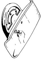
4. Before using, adjust a turning the adjusting knob. needle to zero point by
