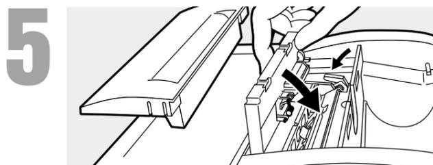
**5 Return the Paper Release Lever, the Automatic Cutter Unit and the Printer Cover to the normal position.**
