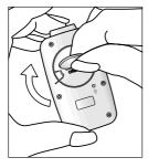
3 Fit the battery cover to the original position, and tighten firmly.
