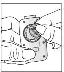
② Set the battery provided (CR2032) with the positive electrode face up.
