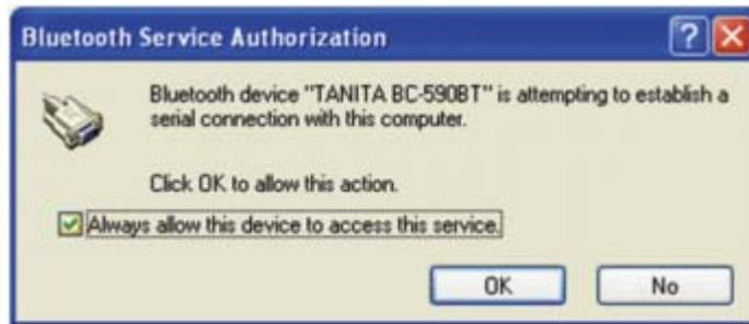
13. The scale is now paired and connected. For future connections, activate the scale (Press Output button on HD-351BT or press a programmed personal key 1-4 on the BC-590BT) and the connection should be made automatically. For verification that a connection is made, the Bluetooth icon in the system tray (lower right corner of computer screen) should change from a white center to a green center.
