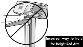
To avoid danger of breaking or coming loose, you must hold the height rod arm securely.
