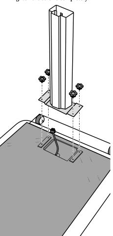
Lower Pillar assembly while carefully inserting the cable into Lower Pillar assembly and extending it the full length of the Lower Pillar.
