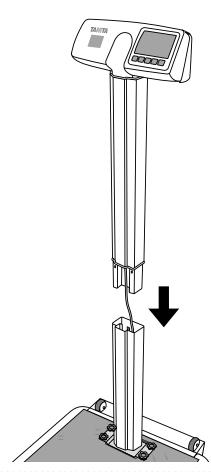
3) Connect the Cable from the bottom of the lower pillar assembly to the cable on the base.
