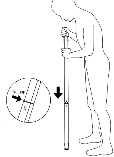
10) Insert the Hight Rod Assembly into the Pillar.
