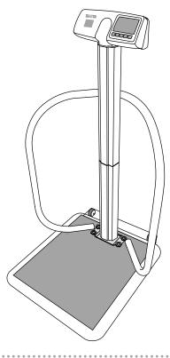
5) Insert the tabs of the brace into the slot. Putting your weight on the handrail to adjust its position will facilitate insertion of the brace into the slot.
