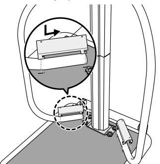
6) Clamp the handrail to the brace using the four screws.
